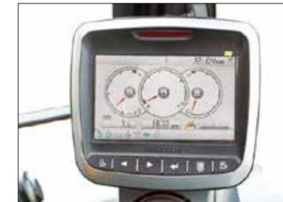
**1** With the installation of a color panel, operators can now easily view equipment operating information ; thus greatly enhancing controllability of the machine.
